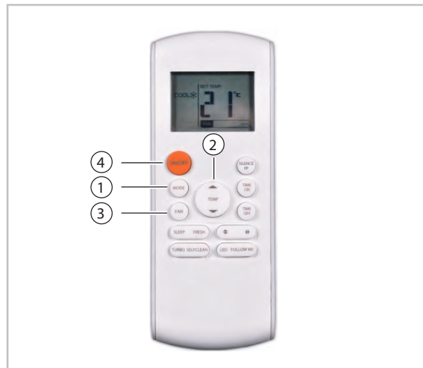
Fig. 19: "Cooling", "Heating" and "Recirculation" mode
